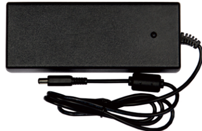
S8-0004 power supply adapter Input: 100~240VAC, 50/60Hz, 1.5A Max. Output: 24V, 5A Max (S8-000405A) 24V, 4A Max (S8-000404A) 24V, 3A Max (S8-000403A)
