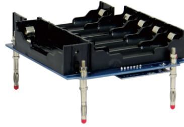
S8-0002 Battery slot 1 Battery slot for S8 series power supply
